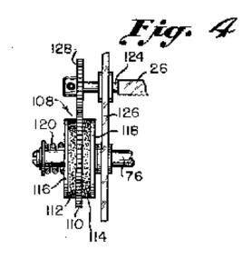
**Two oiled felt disks** 112 and 114 and two Washers 116 and 118, the combination being pressed together with the felt disks bearing against the gear 110 by the force of a compression spring 120.
