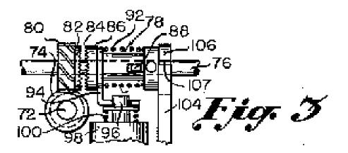
FIGURE 3 is a further detail view of the positive clutch mechanism shown in FIGURE 2 and illustrates the manner in which the sliding clutch member is keyed to the camshaft;
