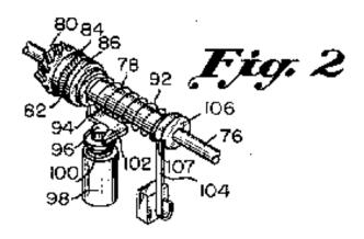
FIGURE 2 is a detail perspective View of the positive cyclic clutch mechanism which can be seen below the typewheel in FIGURE 1 and which controls the camshaft cycles of rotation, the length being exaggerated for purposes of clarity.
