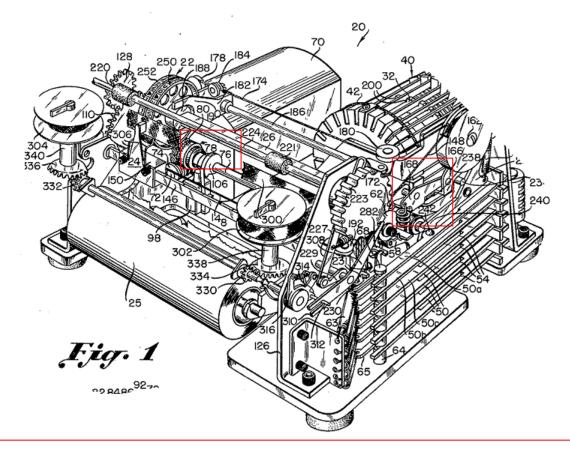
Freely rotatably mounted on the camshaft 76, as the input member of clutch 78,
